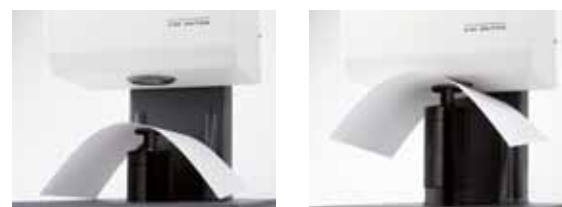
Sample holder – Easier handling of sheet materials
