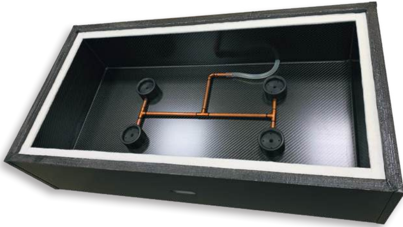
▲ Fig. 7: The heat-cool system HCS-6 exposes the DUT to temperatures from -40 °C to 105 °C.
