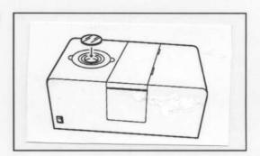
Set the White Calibration Plate into the groove of the Target Mask.
