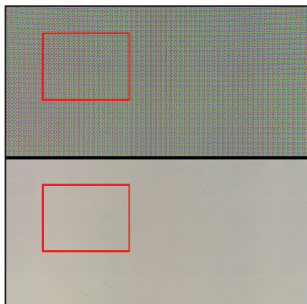
Pre-processing tool Moiré correction in LumiSuite. Upper panel: before correction of Moiré artifacts. Lower panel: with Moiré correction applied. The red square is a zoom in of the blue shaded area.
