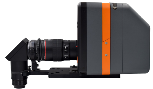
XRE lens with fold mirror, shown with ProMetric I-series imaging colorimeter
