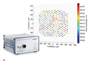
2D peak wavelength analysis of single emitters on a VCSEL array with the VTC 4000 version incl. fiber output. A high-resolution CAS spectroradiometer and an xy-translation stage is required.
