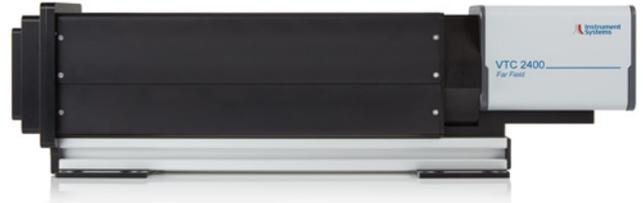
The VTC 2400 is a high-resolution 2D radiance measurement system specifically designed to accurately determine the radiant intensity distribution of VCSEL and LED devices in the far field. It consists of a light-permeable screen with a monochrome camera suitable for measurements in the near infrared wavelength region – fully integrated in a light-proof housing suitable for lab and production applications.
