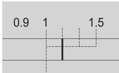
Set in reference of the 1/3 position between the center of 1 and decimal point of 1.5.
