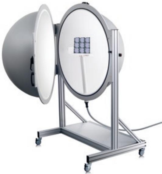
The ISP 1000 integrating sphere with 1 m diameter
