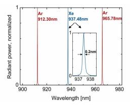
Spectral radiant power of selected Ar and Xe emission lines. They were measured with a CAS 120-HR model with a spectral range of 902 to 982 nm and corresponding spectral resolution of 0.2 nm (FWHM).
