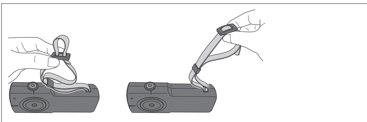
If you will only attach the wrist strap, proceed to step 6 and slide the loop to the strap holder, fixing the strap in place on the strap.
