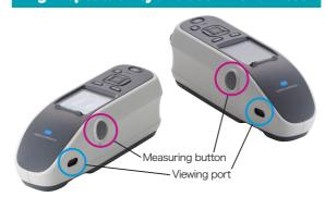
By using a 45°c:0° illumination/viewing system with ringshaped illumination having light sources radially located at certain intervals, the CM-25cG provides stable data while minimizing instrument rotational effects. The system also provides data with high accuracy and repeatability even if there is a small gap between the measurement aperture and the subject.
