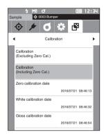
2 Use [▲] or [▼] to move the cursor to "Calibration (Excluding Zero Cal.)", and then press the [Confirmation] key. 3 Set the instrument in the calibration stage in order to measure the calibration stage's white calibration plate.
