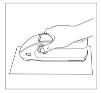
To measure concave surfaces, as shown in the following figure, use the standard flat type battery cover (CM-A218).
