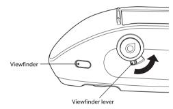
3 As the viewfinder opens, a white LED will turn ON, illuminating the specimen within the range of measurement according to the set measurement area (MAV/SAV).
