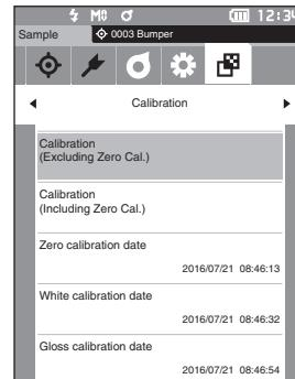
**2 Use [▲] or [▼] to move the cursor to “Calibration (Including Zero Cal.)”, and then press the [Enter] key.**
