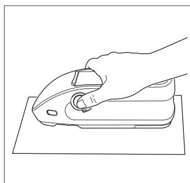
To measure concave surfaces, as shown in the following figure, use the standard flat type battery cover (CM-A218).
