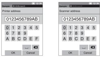
3 After inputting the characters, move the cursor to [OK] and press the [Confirmation] key. The printer/reader will be registered as an I/O device for the instrument, and the display will return to the <Communication setup> screen.
