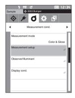
2 Use [▲] or [▼] to move the cursor to "Measurement setup", and then press the [Confirmation] key. The <Measurement setup> screen is displayed.
