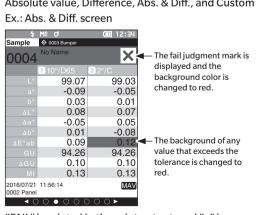
"FAIL" is printed in the print output, and "x" is appended after any value that exceeds the tolerance.
