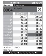
When the number of sample data sets stored in the memory reaches 7,500, "The device memory is full. Please delete some data to measure." will be displayed, indicating that some data sets must be deleted before measurement is possible.
