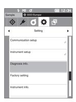
2 The instrument status is diagnosed and the results are displayed.
