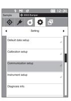
2 Use [▲] or [♥] to move the cursor to "Communication setup", and then press the [Confirmation] key. The <Communication setup> screen is displayed.
