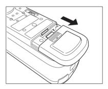
3 Rotate the battery retainer and insert the lithium-ion battery. (Follow the indications in the battery compartment to avoid confusing the battery polarity.)
