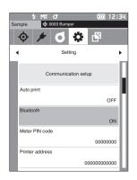
2 Use [▲] or [▼] to move the cursor to "ON", and then press the [Confirmation] key. The instrument's Bluetooth function is turned ON and the display will return to the <Communication setup> screen. The Bluetooth icon will be displayed in the status bar. To configure the Bluetooth PIN code, go to step 3 to
