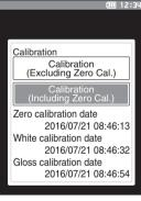
3 Set the instrument in the calibration stage in order to measure the calibration stage's white calibration plate.
