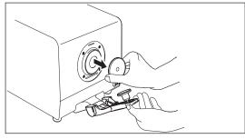
3. Take the desired target mask in your hand, and attach it to the CM-3600A. Make sure that it fits into the concave area around the integrating sphere opening.
