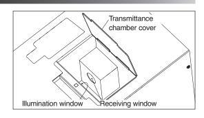
**3.** Close the cover of the transmittance chamber.
