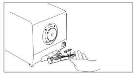
2. Position the white calibration plate so that it is held in place by the sample holder by fitting the sample holder pad into the concave (rear) side of the white calibration plate as shown at right.
