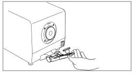
2. Fit the projections of the zero calibration box into the grooves on the CM-3600A and then close the sample holder to hold the box in place.
