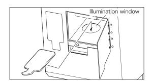
3. Close the cover of the transmittance chamber.
