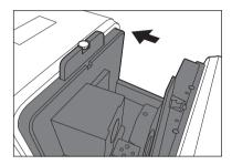
2 Install the transmittance zero calibration plate in a position so that it completely covers the illumination window.
