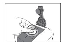
2 Fit the Zero Calibration Box into the indentation on the instrument.
