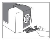
2 As shown in the figure, press on the sample holder so that the sample holder fits into the indentation on the reverse side of the white calibration plate.
