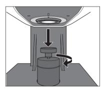
2 As shown in the figure, fit the sample holder into the indentation on the reverse side of the white calibration plate and return the sample holder to its original position.
