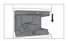
2 Directly slide the cover closed so it closes securely. The cover is locked when it is closed to the point where it clicks.
