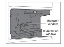
3 Close the transmittance specimen chamber cover.
