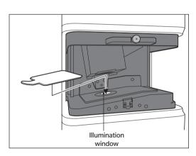
3 Close the transmittance specimen chamber cover.
