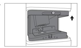
2 Install the transmittance zero calibration plate in a position so that it completely covers the illumination window.
