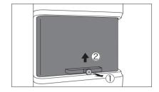
2 Under those conditions, slide open the cover until a click sound occurs and it fits into place. The cover is fastened at the top by magnets.
