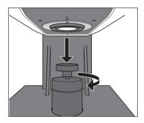
2 As shown in the figure, fit the sample holder into the indentation on the reverse side of the gloss calibration plate and return the sample holder to its original position.
