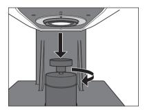
2 Fit the concave part of the zero calibration box onto the sample holder and return the sample holder to its original position.
