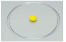
Pastes can also be measured using a Petri dish (optional accessory).
