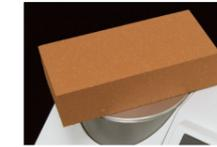
By using the Ø3 mm target mask (optional accessory), even small samples can be measured.
