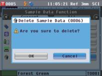
2. Use the button of the cross key to move the cursor to "OK" and press the [OK/Edit] button. The data is deleted.
