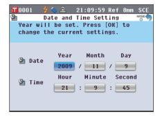
2. Use the or button of the cross key to move the cursor to a desired item and then press the [OK/Edit] button.
