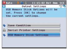
3. Use the or button of the cross key to move the cursor to "Serial Printer Settings" and then press the [OK/Edit] button.
