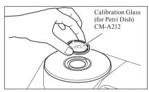
4. Align the White Calibration Plate with the positioning groove on the Target Mask for Petri Dish and push the plate in.
