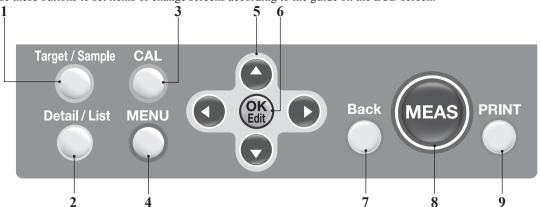
1 [Target/Sample] button Switches between <Target> screen and <Sample> screen.
