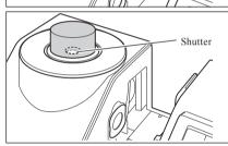
4. Look into the Specimen Viewing Mirror from the Top and adjust the position of the specimen.
