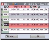
4. After all desired targets have been selected, use the ♠ or ♠ button of the cross key to move the cursor to the "OK" button and then press the [OK/Edit] button.
