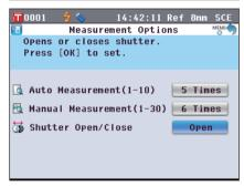
Memo For the transmittance measurement, the geometry will be set to di:0° when the shutter is closed and will be set to de:0° when the shutter is open and the Zero Calibration Box is set.
