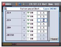
4. When you finish all settings, press the ▶ button or [MENU] button of the cross key to move the cursor on "Save", and then press the [OK/Edit] button.
