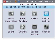
2. Use the or button of the cross key to move the cursor to calibration options and then press the [OK/Edit] button.
