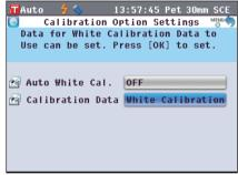
3. Use the or button of the cross key to move the cursor to the desired calibration data and then press the [OK/Edit] button.
