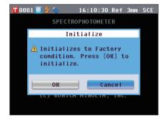
2. Use the **③** or **⑤** button of the cross key to move the cursor to "OK" and then press the [OK/Edit] button.
