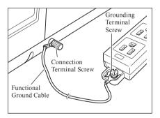
2. Connect the other Y terminal of the Functional Ground Cable to a reliably grounded object (e.g. a 100-240 VAC earth terminal or a metal desk).
