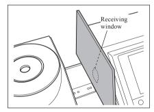
4. Open the shutter and blow off the dust and dirt in the Integrating Sphere with a blower.
