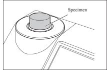
3. Make sure that \$\frac{1}{2}\$ (Ready to measure) is displayed and then press the measuring button.
