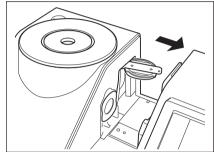
3. Block the receiving window of the Transmittance Specimen Chamber so that no dust or dirt enters through it.
