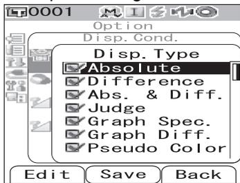
For example, when the screen shows the guidance **Edit** **Save** **Back**, the [SAMPLE], [SAVE/SEL] and [TARGET] buttons are assigned with the Edit, Save and Back functions respectively. In this manual, when the button name and the function assigned to the button are different, the button name and function are described as “the [SAMPLE] (Edit) button” or “[TARGET] (Back) button”.
