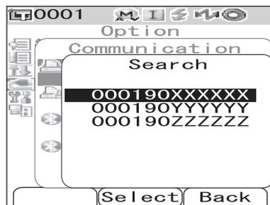
**5 Use the  $\Delta$  or  $\nabla$  button of the cross key to move the cursor to the Bluetooth address of the printer.**
