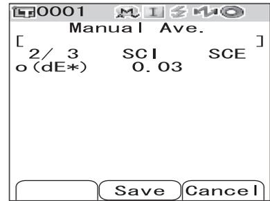
**4 Place the specimen measuring port at the next position and repeat the steps from 1 to 3.**
