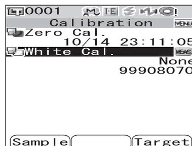
**3** If necessary, use the  $\nabla$  button of the cross key to move the cursor to “White Cal.”
