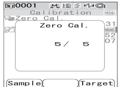
When zero calibration is finished, the screen returns to the <Calibration> screen.
