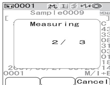
When the specified number of measurements has been completed, the averaging result will be displayed on the screen.
