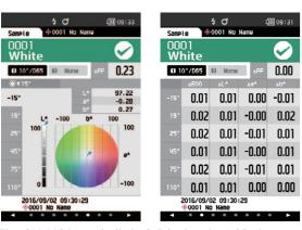
The CM-M6 has a built-in 3.5-inch color LCD that can display measured values both numerically and on colored graphs, for easier visualization of results.
