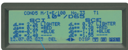
Simultaneous color difference with wording for SCI and SCE Relativity Gloss Value
