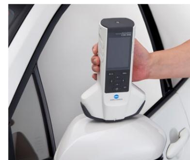
The viewing beam is 6 mm in diameter, so small surfaces that were hard to measure with earlier models can be stably measured.
