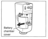
2 Install four AA-size batteries in the battery chamber with the polarities as shown inside the chamber.
