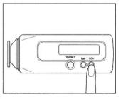
3 Place the tip of the Color Reader flat against the color chosen as the target color and press the measuring button. When measurement of the target color has been completed, a beep will sound and the display will change to the target color display, showing the results for the target color measurement.
