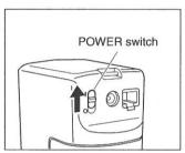
2 Set the POWER switch of the Color Reader to I (on) and then switch on the printer.
