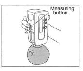
If a mistake was made in measuring the target color, press TARGET to return to the target color measurement display and repeat the above procedure from step 2.
