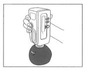
The color space in which the results are displayed can be changed after measurement by pressing Lab (for L\*a\*b\* color space) or LCh (for L\*C\*h color space).
