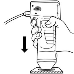
**5 Press the Measure/Enter key**
