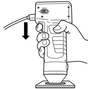
**10** Press the Measure/Enter key
