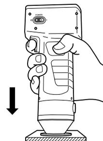
**4 Press the measurement button after making sure the ready lamp is ON.**
