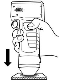
**4 Press the measurement button of the measuring head after making sure the ready lamp is ON.**
