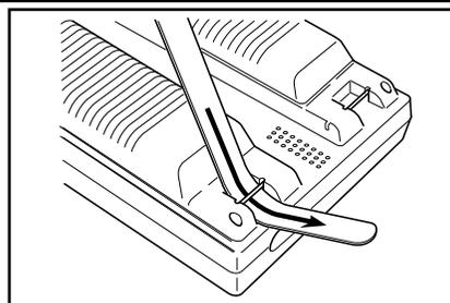
**2** Pass the strap back through, as shown in the figure at right.
