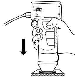
**6** Press the Measure/Enter key
