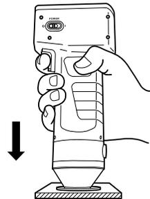
**2 Press the measurement button of the measuring head after making sure the ready lamp is ON.**
