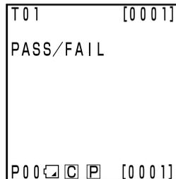
O PASS: This is displayed when the value is within the color difference tolerance.
