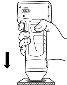
**2** Press the measurement button after making sure the ready lamp is ON.
