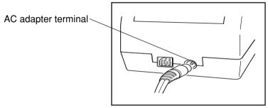
nsert the AC adapter power plug to an AC outlet (100-240 Vac).
