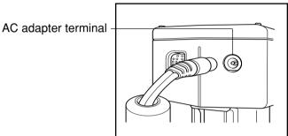
Insert the AC adapter power plug to an AC outlet (100-240 Vac).
