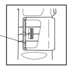
2 Insert 4 AAA size batteries in accordance with the polarity indications shown in the battery chamber.
