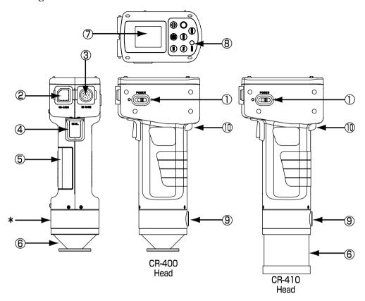
1. Power switch : Turns ON and OFF the power.
