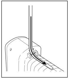
**7** Pass the strap back through, as shown in the figure at right.
