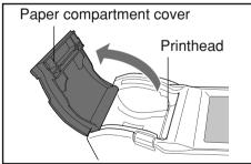
2 Load the roll paper so that it is oriented as shown in the illustration, and pull the paper out so that about 3 - 4 cm of it extends over the paper cutter.
