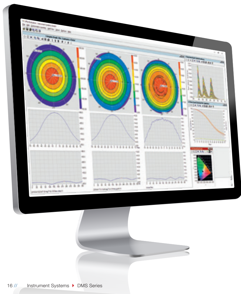
Fig. 15: The Flicker Graph view shows luminance fluctuations of a photometer measurement as a function of time, FFT flicker luminance and VESA resp. JEITA flicker curves as a function of wavelength and flicker evaluation results.
