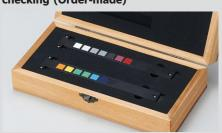
Color tiles enable users to easily check that the measurement values from their FD-9 are correct.
