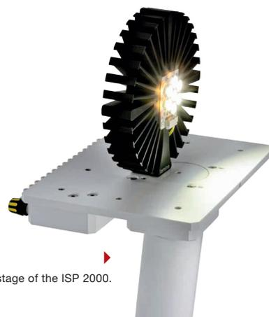
A sample stage can be used instead of the lamp post for mounting non-standardized test specimens, such as complete luminaires and LED modules. This platform offers a base measuring 200 mm x 150 mm with variable height adjustment and a 16-pole terminal strip for controlling and monitoring the test specimen. A version of the sample stage is supplied for test objects with prefabricated connecting cables. The cable is routed to the outside of the
