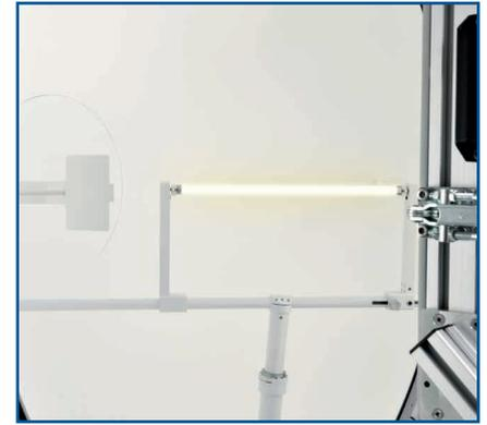
▲ Sample mounts for linear tubes with G13 socket.
