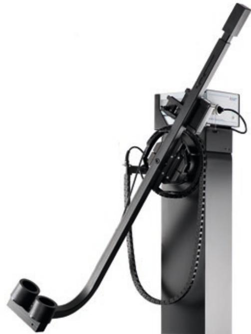
Luminous flux integrator with photometer and spectroradiometer
