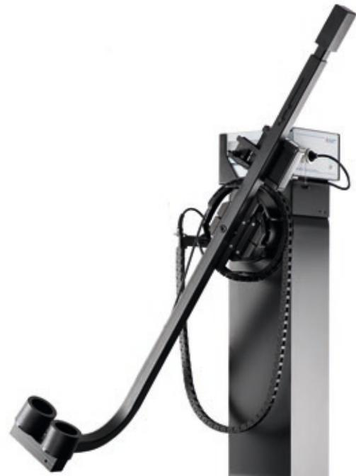
Luminous flux integrator with photometer and spectroradiometer
