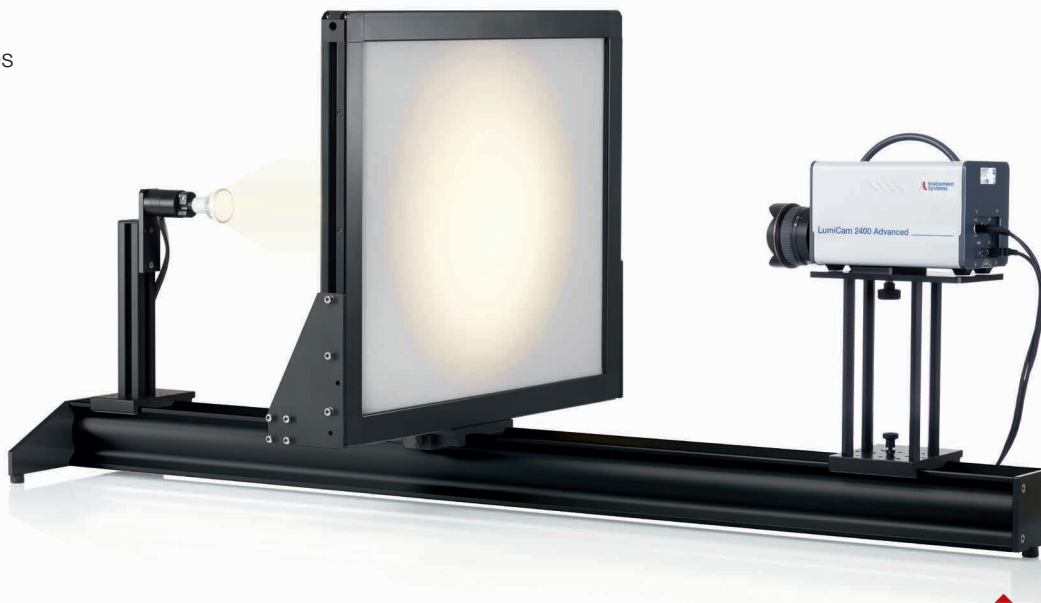
The LVK analysis kit comprises a LumiCam, a light permeable screen and a light source.
