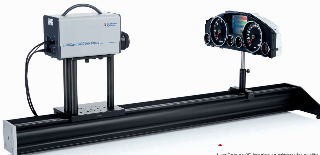
▲ LumiCam as 2D imaging colorimeter for quality assurance of dashboards in automotive industry.
