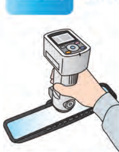
Spectrophotometer CM-700d (For surface reflectance measurement)
