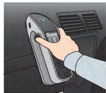
Spectrophotometer CM-25cG Gloss (Color control of parts with differing textures)
