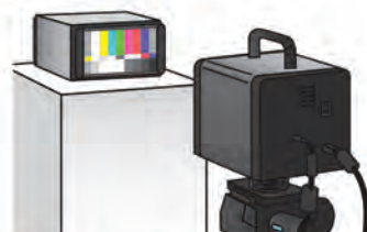
2D luminance colorimeters CA-2500A LumiCam2400B Color/Advanced (For black mura evaluation)
