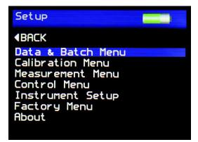
The Setup Screen is used to customise the instrument to the user's preference. Pressing the Up and Down buttons navigates through the options, pressing the Enter button selects that option.
