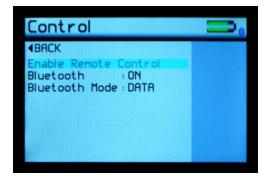
3. If the Bluetooth icon is not visible, enable it as detailed in Control Screen. Ensure that Bluetooth mode is set to either Data or Data+
