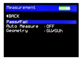
The Measurement Screen is used to configure the instrument's measurement parameters to the user's preference. Pressing the Up and Down buttons navigates through the options, pressing the Enter button selects that option.
