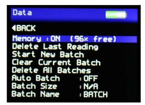
The Data & Batch Screen is similar in functionality to that of the menu screen but also allows the selection and setting of the Auto Batch size.
