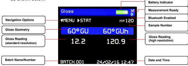
In this mode, measurements can be made by simply pressing any of the measurement buttons.
