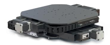
The SCAN 300 x-y scanning stage is an optional accessory for use with DMS systems DMS 803, DMS 505 and DMS 201. This motorized positioning stage extends the existing x-y travelling range of the basic mechanism of the DMS 803 and the DMS 505 to 300 mm x 300 mm allowing full scans of displays up to 16". Moreover, it enables motorized positioning and automated scanning with the manual DMS 201 system.
