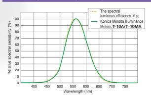
Ideally, the relative spectral responsivity of the illuminance meter should match V ( $\lambda$ ) of the human eye for photopic vision. As shown in the graph above, the relative spectral responsivity of Konica Minolta Illuminance Meters T-10A/10MA is within 6% (f1) of the CIE spectral luminous efficiency V ( $\lambda$ ).
